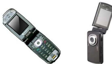
Fig. 6. Fingerprint mobile phone ('L' company) and facial recognition mobile phone ('S' company)
